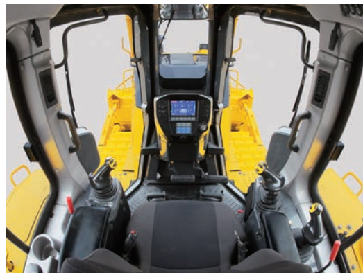
Fully suspended operator station ensures maximum operator comfort and an excellent view on the blade.
