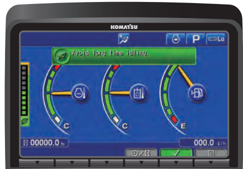
The ECO-gauge, the new fuel consumption gauge, idle caution and auto idle stop function all assist to further reduce fuel consumption.
