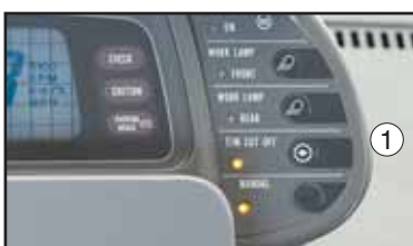
1. T/M cut-off ON/OFF switch 2. T/M cut-off set switch
