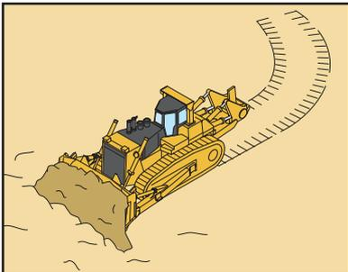
When dozing and turning, the ECMV automatically controls the stroke ratio of the steering clutches and brakes, depending on degree of load, enabling smooth dozing and turning.
