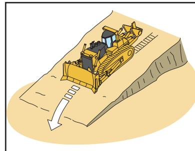
When dozing downhill, the ECMV automatically controls the steering clutches and brakes depending on incline of the machine or degree of load, reducing counter-steering and enabling smooth dozing operations.
