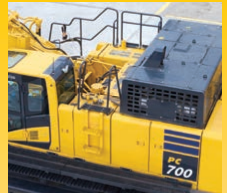
Hand rails and anti-slip plates
