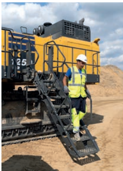
The standard hydraulically operated stairway provides safer access and egress to and from the machine.
