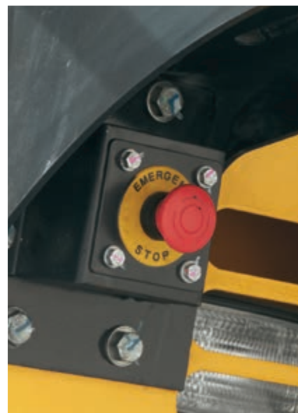
Three emergency engine stop switches are installed in the cab and around the machine, as standard.
