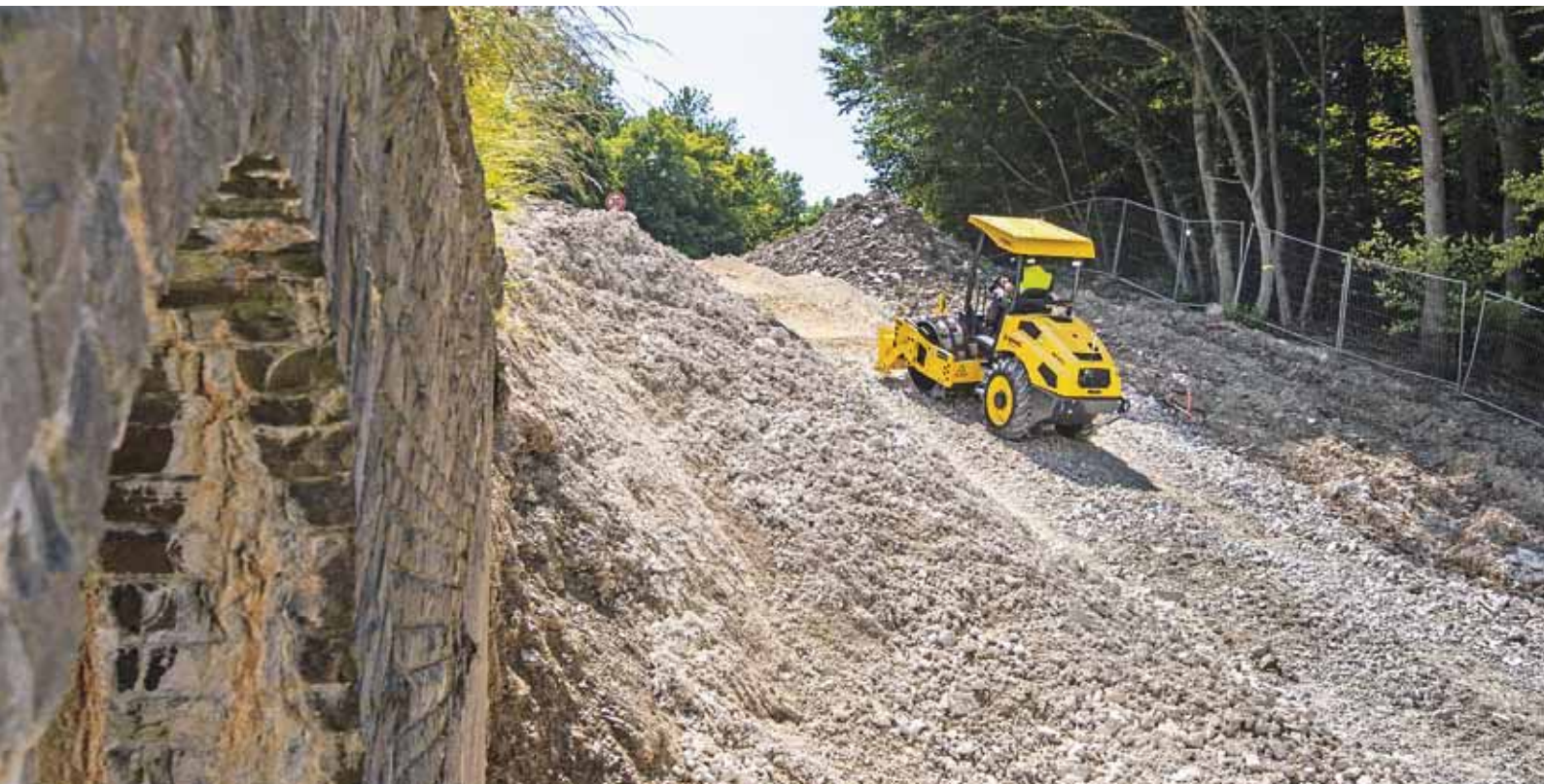
DH With a gradeability of up to 64%, double-pump models meet the toughest demands.
