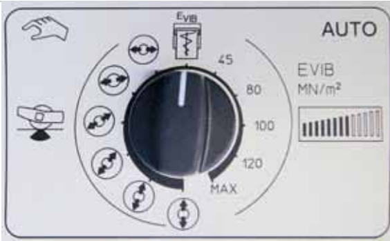
Easier: VARIOCONTROL operation with a single switch.
