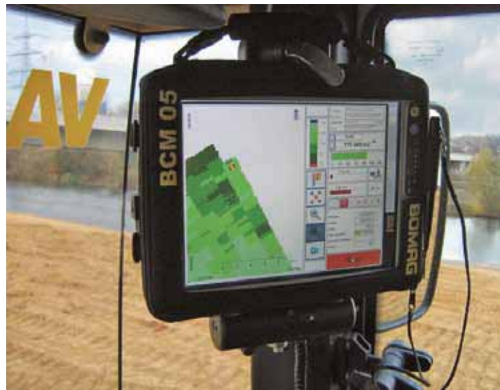
Continuous dynamic compaction control with BCM 05.
