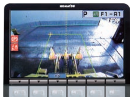
Fully integrated rear-view camera system
