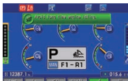
Eco-gauge, Eco guidance and fuel consumption gauge
