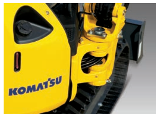
The swing cylinder has been relocated to the left hand side of the excavator to minimize protrusion so the operator doesn't have to worry about the cylinder when working near a wall.
