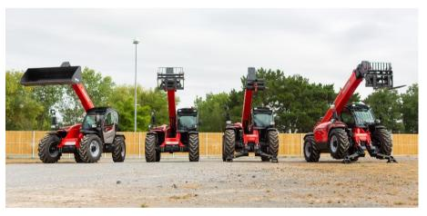
The 11 meters and 13 meters models are available with two transmission versions, torque converter or hydrostatic, to meet the different needs of users. Two engines are also available for these same models, a 75 hp version or a 100 hp version. These telehandlers are thus equipped with the same dashboard as the rest of the range, with a Harmony screen, as well as the option to move its control buttons to near the armrest (Double Switch Buttons).
