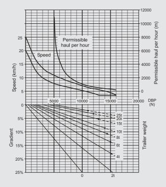
Load/gradient combinaisons shown by full line can be restarted from stationary on the gradient. The permissible haul per hour is the total distance travelled, including the return journey and any downhill gradients.
