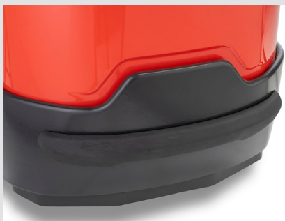
Front casted steel bumper
