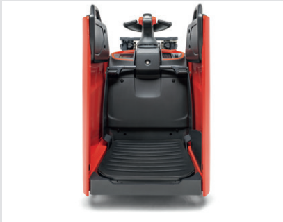
Steel chassis to protect the driver
