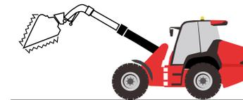
**Automatic return to load:** to easily return to a position (attachment and boom) pre-determined by the operator. This function is particularly useful for loading operations.
