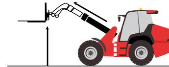
**Bucket shaker:** quickly empties the bucket without requiring the operator to make repetitive movements. Manure will no longer stick to the bottom of the bucket.
