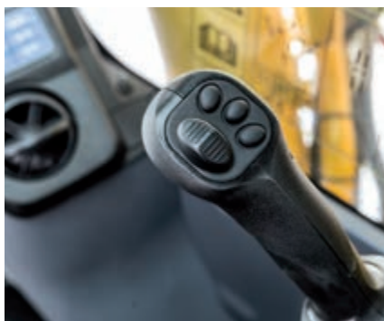
Joysticks with proportional control button for attachments
