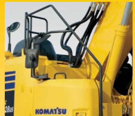
Hand rails and anti-slip plates
