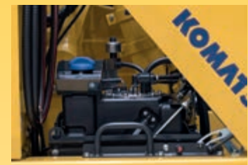
Simple access to the AdBlue® tank
