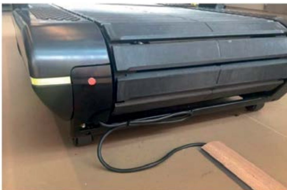
Fig. 11 - Layout 5 OK but the use of a cable sheath is recommended
