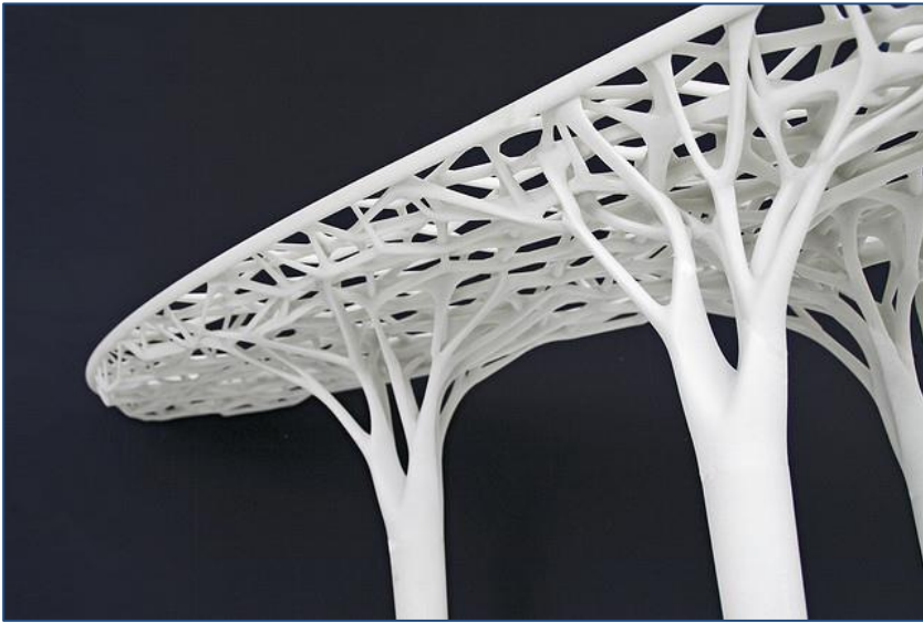
Figure 4: 3D printers can construct geometrically highly complex models. The illustration shows an extract from "The Trabecula Bench". The bench is 36 cm in height with a length of 180 cm, and the bench's structure is based on that of bird bone.
