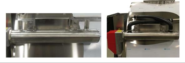
Installation of the heater at the front of the tank to/at the Argos console
